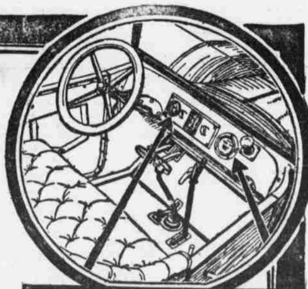
Speedometer, fuse box, ignition, lights, battery regulator, all mounted flush on instrument board.
