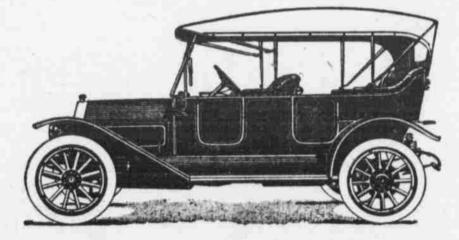
· 4½x5½ Motor, 120-inch Wheel Base 36x4 Tires, Full Floating Rear Axle.
