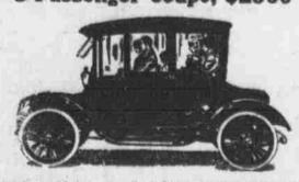
Wheel base 96 ins., comfortable seats for five, all facing forward: Borland patented horizontal control, from either forward or rear seat; six forward and three reverse speeds; automatic cut-out disconnects power when emergency brake is applied. "Exide" batteries, standard equipment. Luxuriously equipped with every need and convenience. A roomy, comfortable car for all the family.
