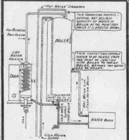
DOTTED PIPES = ( ) SHOW CIRCULATION OF HOT WATER. SHORT LINES IN PIPES = ( ) SHOW ECIRCULATION
