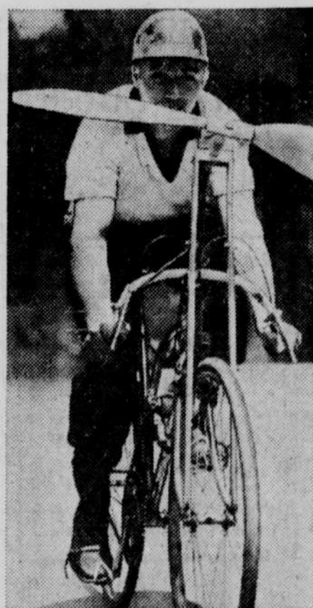
The addition of a propeller which controls the speed of his streamlined "aerocycle" makes it possible for Dominick Devincenzi of Chicago to drive his bicycle at the rate of 45 miles per hour.
