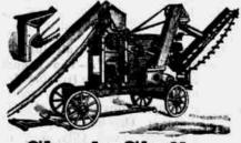
Shuck Sheller. Only one made that successfully shells corn with the shuck on as well
