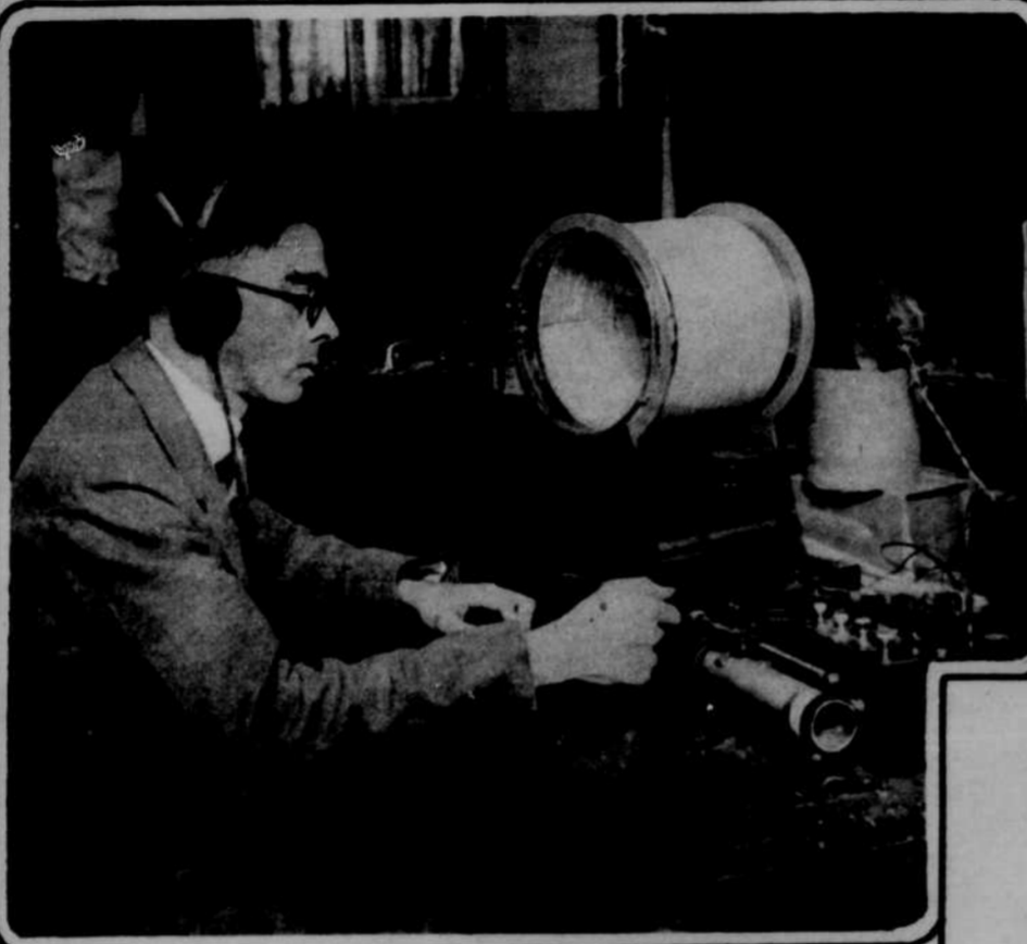
An air policeman, M. S. Strock of the Bureau of Standards, Washington, D. C., measuring the wave lengths or frequencies of American and European code transmitting stations for use as standards. The government checks up on the broadcasting stations to see that they use wave lengths assigned them. Wide World
