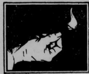
A match held in the air on a pin will burn completely. LAW NO. 3— Oil Must Be Mixed With Air.
