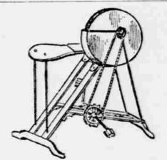
GRINDSTONE WITH PEDAL GEAR,
