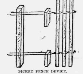
wire tight. Put a picket between the wires and turn the blocks over as often as you wish to twist the wire between each picket; then put in another picket and twist the other way, etc. To preserve posts, mix pulverized charcoal in boiled linseed oil to the consistency of paint and apply with a brush.
