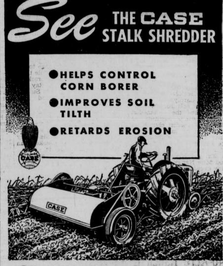
Thoroughly shreds corn, cotton and other crop residues. Quickly prepares ground for clean plowing-faster and easier than disking. Shreds up to 25 acres per day under favorable conditions with ample power. 84 long-wearing chain-attached swinging hammers deliver 1900 shredding blows per second. Shreds an 80-inch strip. Adjustable ground clearance. Heavy-duty throughout-sealed gears run in oil bath, strong tubular frame, anti-friction bearings. Come in and see this fine shredder.
