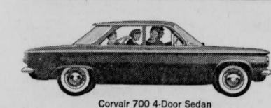
If you haven't driven it yet, you don't know what a delight driving can be. Its steering, response, traction and roadability are unique because it's a unique car -the only U.S. car with an air-cooled airplane-type rear engine, transaxle and independent suspension at all four wheels. Be in on the know.
