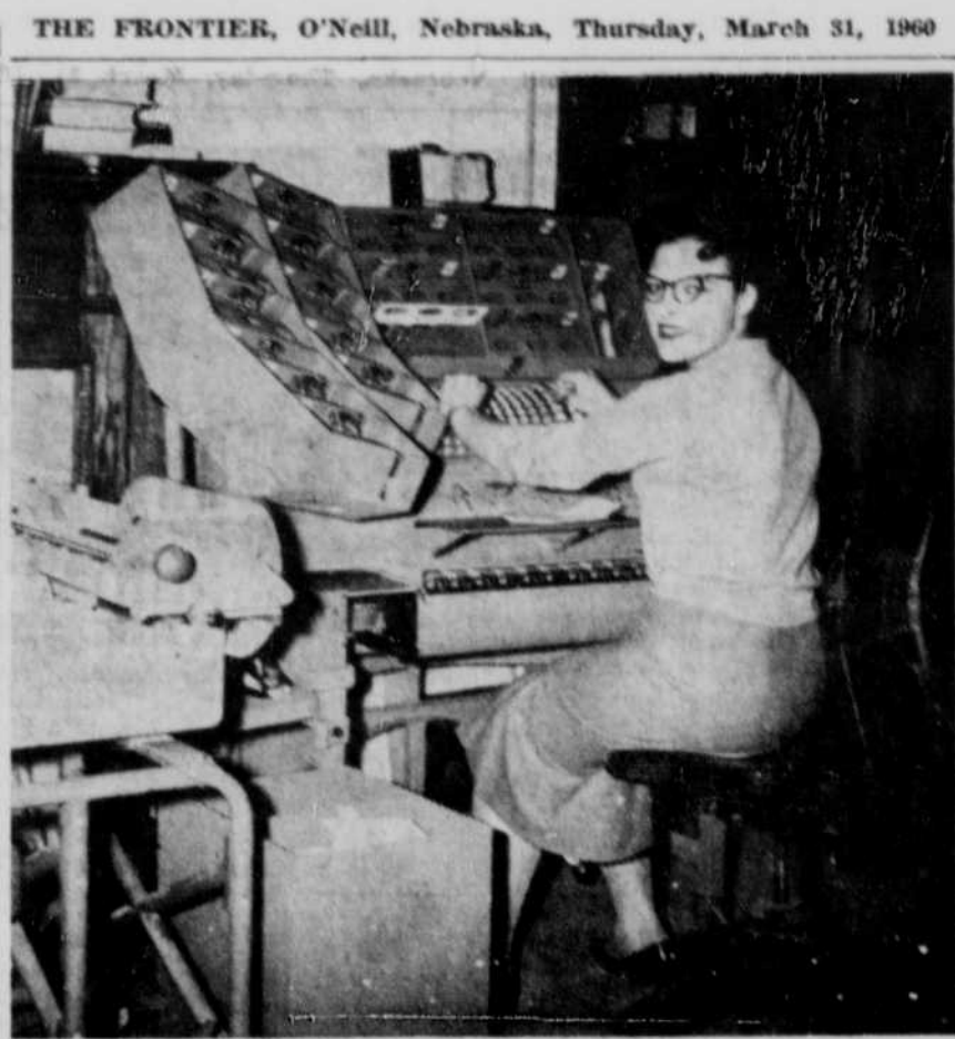
Ellen Havranek sits at a new accounting machine installed at the O'Neill National bank during the past week. The machine rough sorts checks and deposit slips and keeps a tabulation of all bank transactions.
