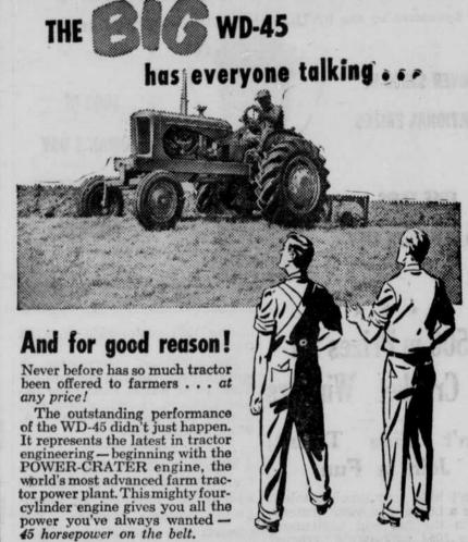
Yes, and there's more. Complete hydraulic system with automatic Traction Booster, built-in, two-clutch power control, Power-Shift rear wheels, plus the newest of all — the SNAP-COUPLER... team up to bring you a combination of conveniences that get all farming jobs done easier... faster — unmatched in any other farm tractor... as
