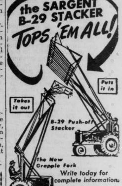
The SARGENT 8-29 ( Is the highest tractor mounted stacker on the market 29 feet reach with pushoff. 21 feet The famous hydraulic tooth control gives you positive, balanced control of all attachments at all time
