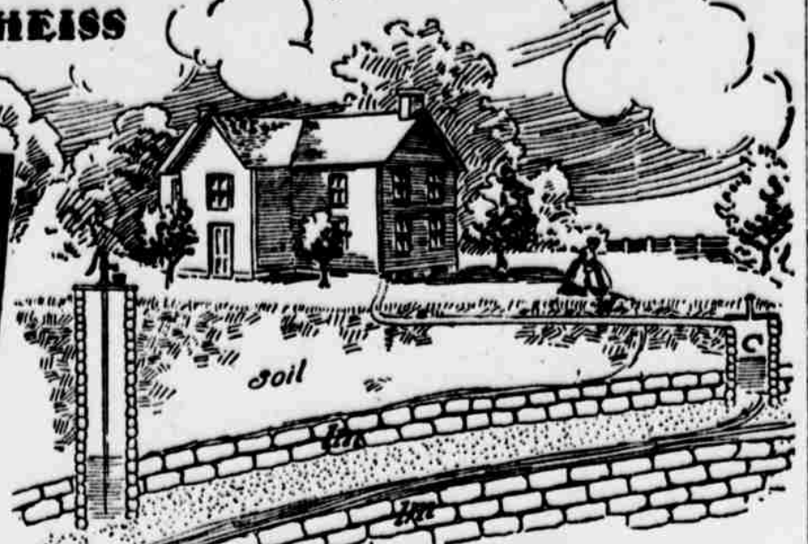
SHOWING HOW DISEASE GERMS OFTEN REACH DRINKING WATER. C. CESSPOOL 7TH. LAYER OF ROCK W. WASHWATER
