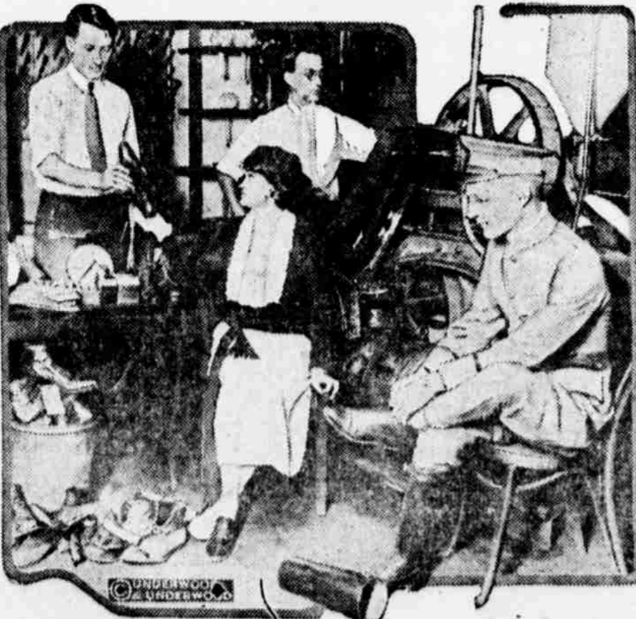
Actual wear tests on army and civilian leather are compared with machine tests in the bureau of chemistry of the Department of Agriculture, where machines are being developed to measure the wearing quality of sole leather. R. W. Frey, in charge of leather work, is shown at one of the machines.
