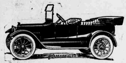
An ideal family vehicle at a price that places it within reach of anyone. Plenty of room for five and plenty of power for any load. Wheel base 106 inches, 32x31/2 tires, anti-skid in rear, 28 brake test H. P., complete electric equipment. Delco system, new windshield, inside top curtains, and every other feature necessary to make it a car for the family.
