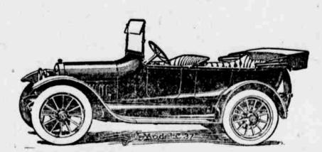
A beautiful steamline body, with graceful cowl; extra wide deep seats, advanced ideas in design and every detail making for utility, places this car at once in a class of its own. 35 actual brake test H. P., 34x4 tires, anti-skid in rear wheel base 112 inches. Full Delco equipment for starting and lights. Inside curtains, new shield and every feature of notable excellence.
