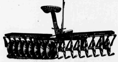
The above cut shows our Budlong Disc Harrow. Owing to several points of construction this harrow will work easier and and more evenly in all kinds of soil than any other: First, because the harrow is FRAME-LESS; second, the gangs are attached to the cross-bar and inner draw-bar, which give it direct draught and make a perfect under-hitch. This gives the gangs a FLEXIBLE movement.
