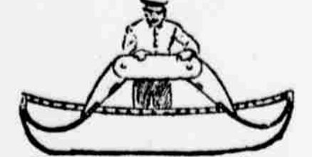
Device to Prevent a Collapse. The spring ribs attached to the stem and stern of the boat. The picture shows the operation of inserting these ribs in the sleeves and springing one of the braces down into the bottom of the boat. When once in place they not only stiffen the craft from stem to stern, but also offer considerable pressure on the ribs which bear the cross-strain when the boat is in the water. To fold the boat it is necessary to exert considerable pressure on the central sections, which must be elevated and the motion reversed to withdraw the end ribs from their places in the sleeves.
