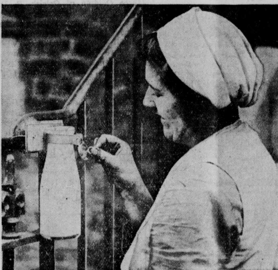
Thieves will find it difficult to get away with milk if this idea evolved by a Rochester, England, resident becomes popular. The anti-milk thief device consists of two hinged clips and a small padlock. The milkman has one key, the duplicate is held by the wife of the man who invented the gadget.
