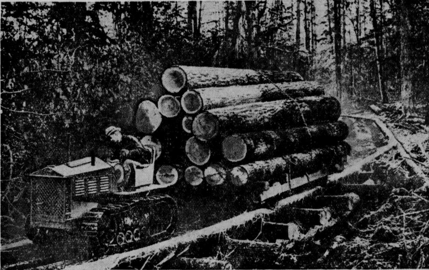
Heavy power machinery and other mechanical equipment has largely revolutionized logging methods in the past decade. An example is in the Naylor logging camp near Ravensdale in western Washington. A 110-horsepower caterpillar tractor is able to pull a 10-ton load of logs on a flat car which runs on wooden rails. Huge logs are thus hauled a distance of more than two miles, from where the trees are felled to the saw-mill.
