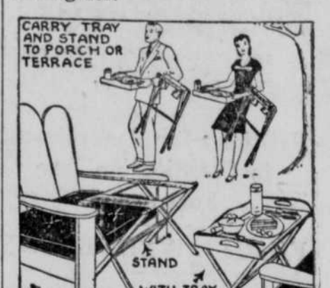
The folding stand is the right height to use with comfortable chairs, and the plywood tray with a gallery around three sides and hand-hold openings, fits securely over this base. The construction of both pieces is so simple that you will want to make a number of them.
