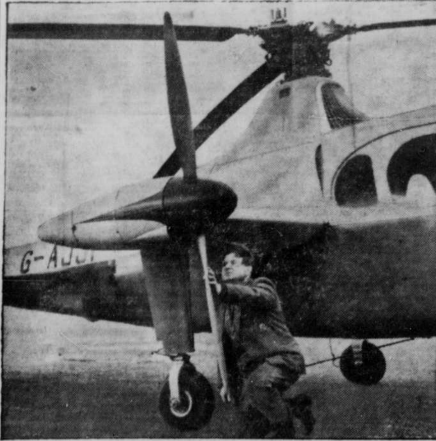
'AUXILIARY' HELICOPTER ENGINE . . . This new Faircy Gyrodyne helicopter has a stub wing with a propeller that provides most of the forward propulsion, while the main rotor keeps the aircraft aloft. The rotor aircraft has a cruising speed of 115-120 mph., and is said to be ideal for intercity flights, air charter work and crop spraying.
