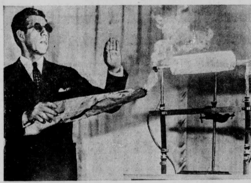
S. G. Hibben, director of applied lighting at the Westinghouse lamp laboratories in Bloomfield, N. J., shown with the 10,000-watt mercury vapor lamp that produces a light one-fifth as bright as the surface of the sun. Although encased in a cooling jacket of running water, the radiations from the lamp set fire to the wrapping paper.
