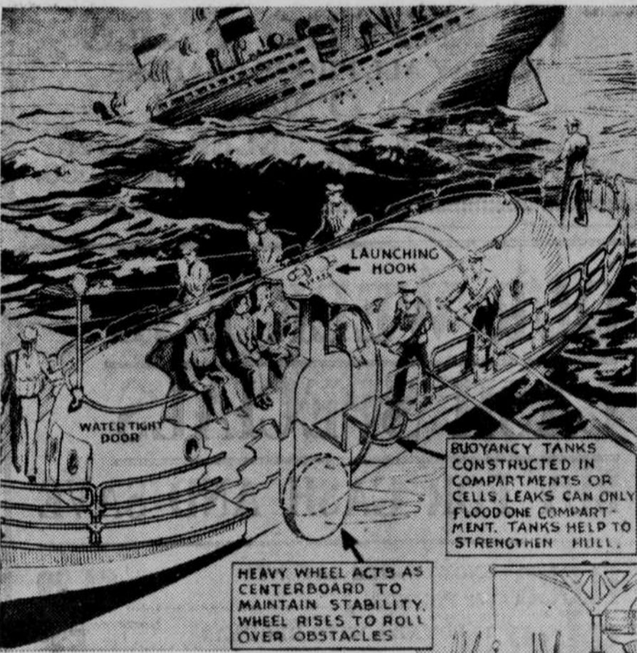
The invention of William L. Wheeler, Los Angeles, Calif., this lifeboat is claimed to be unsinkable. He invented the boat after three of his family had been lost in sea disasters. It is all enclosed, making it non-sinkable and non-capsizable. Buoyancy tanks underneath help keep it on an even keel. Designs for the boat have been completed by a famous artist, and application has been made for a patent.
