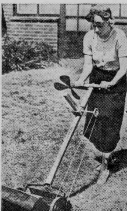
Hot weather hint: This resident of Kent, England, attached the blades of an old electric fan to the lawn mower. By means of a few gear wheels the fan revolves, blowing a cooling breeze as soon as the machine is pushed along the grass.
