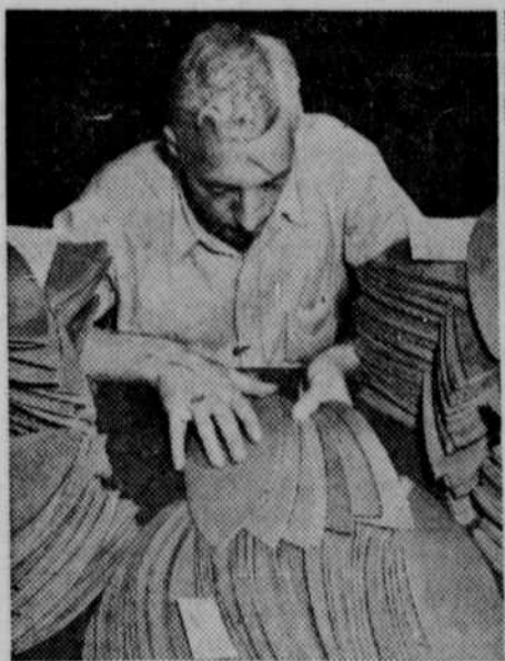
LEFT—Panels are examined still more before a skilled craftsman matches them, guaranteeing that the finished football will have uniform color and quality. RIGHT—The assembly job begins when panels are stitched on a hot wax machine.
