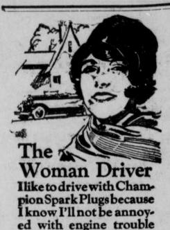
due to faulty spark plugs. Champion is the betterspark plug because it has an exclusive sillimanite insulator specially treated to withstand the much higher temperatures of the modern high-compression engine. Also anew patented solid copper gasket-sealthatremains absolutely gas-tight under high compression. Special analysis electrodes which assure a fixed spark-gap under
