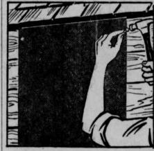
Apply the sheets vertically. Begin the nailing in one corner. Then straighten out the roofing sheet, stretch it horizontally and allow it to hang smooth. Nail from the top down on both sides, stretching the roofing as you go along. Nails should be alternated, one side and then the other, and the roofing should be allowed to hang free with no attempt to distort or shape it.
