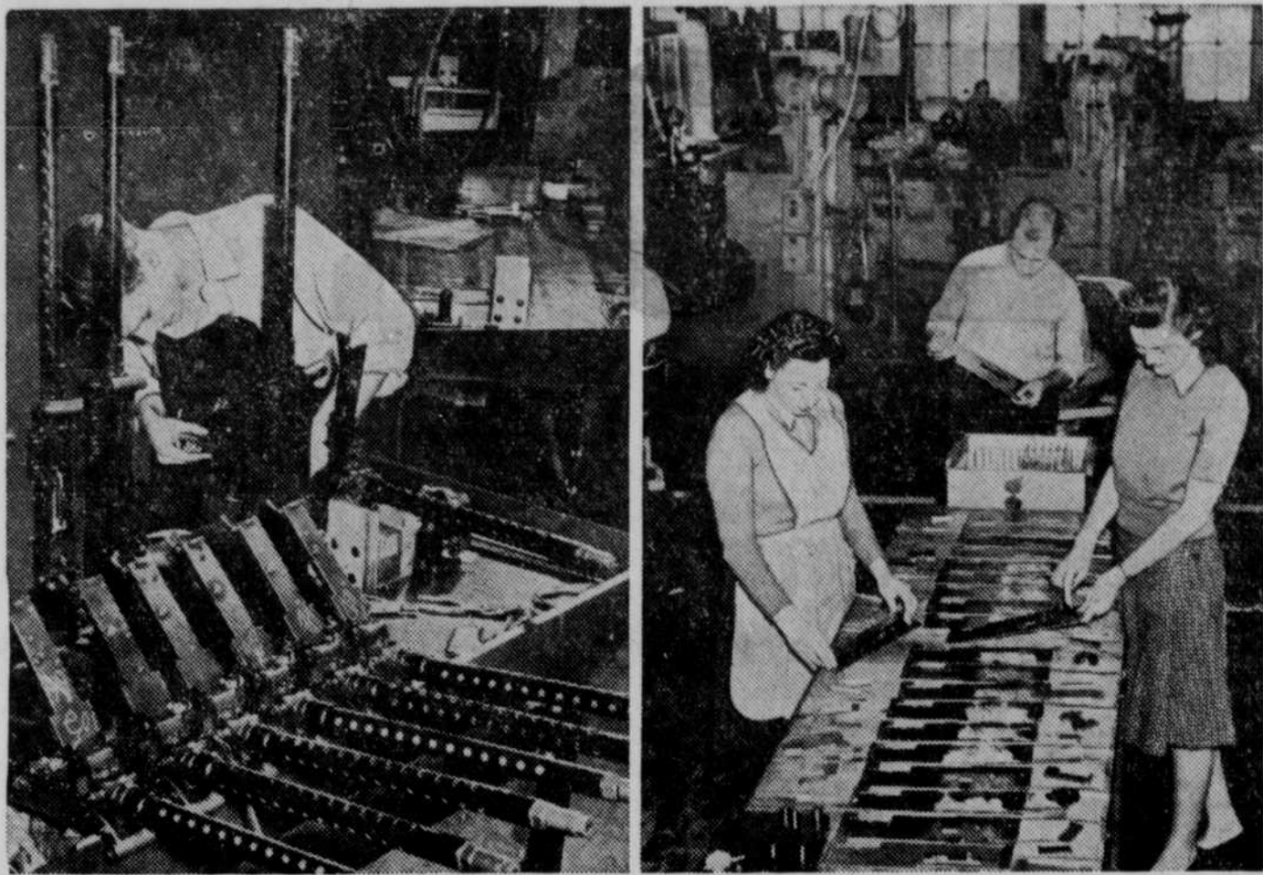
Machine guns sprout where auto parts once grew in the Brown-Lipe Chapin division of General Motors in Syracuse, N. Y. Above at left you see an inspector putting the final Okay on a bevy of Browning machine guns before they are taken to the test range for inspection. At right, machine gun slide plates are carefully checked to .002 of an inch. There are about 300 parts in each machine gun turned out here.
