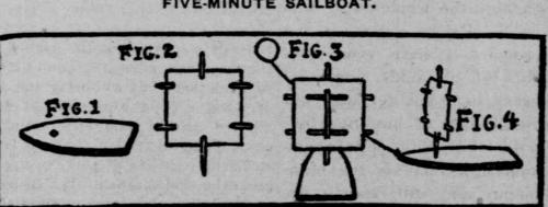
Diagram of Boat's Construction.
