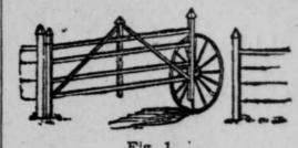
remaining two. The gate rests on the wheel, whether closed or open, the revolving wheel carrying the gate around whether opening or closing. The gate rests on the back end on a block of wood, in which there is a socket, and in this a gudgeon at the foot of the gate head rests and turns. Mr. Scott says his three-year-old boy can open an 18-foot gate of this sort with ease.
