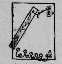
has a radius of 4 inches. Place the contact screws along this arc and about 1/2 inch apart, center to center; the last screw forms a part of binding post A.
