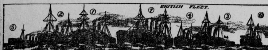
BRITISH FLEET—(1) Cruiser Indefatigable, 3,600 tons, 44 guns; (2) cruiser Retribution, 3,600 tons, 22 guns; (3) cruiser Charybdis, 4,360 tons, 30 guns; (4) sloop of war Albert, 350 tons, 6 guns; (5) torpedo boat destroyer Quail, 300 tons, 6 guns; (6) cruiser Tribune, 3,400 tons, 22 guns; (7) cruiser Ariadne, 44 guns.
