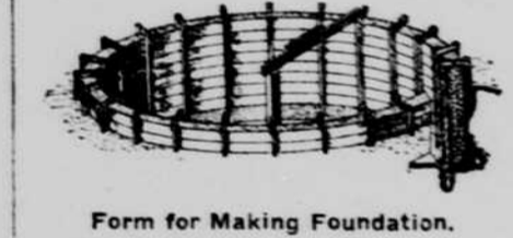
Form for Making Foundation.
