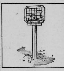
desired point which serves to indicate the location of said guide-board in the particular district or township delineated by the map on its face. The guide-board has a border on which are inscribed names of towns and other locations lying outside the one in which the guide-board itself is located, and also the distances of such towns and locations from points indicated on the map proper.
