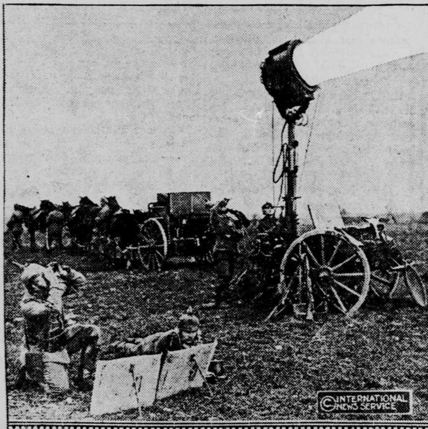
One of the German field searchlights which are so useful in observing against attacks from the air. The officer in the left foreground is observing an enemy aeroplane, his instructions being sent by the telegrapher at his side to the nearest artillery position.
