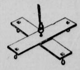
one small windlass. I have used this for several years and find it quite satisfactory. Stock is watered from this well. A pump is placed close to the wall, and as the well is large one does not interfere with the raising or lowering of the milk pails.
