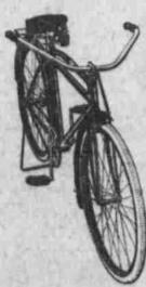
It has a 20-inch Frame with Coaster Brake. Motor Bike Handle Bars, Eagle Diamond Saddle, Motor Bike Pedals, Motor Bike Grip, Luggage Carrier Holder, Folding Stand, Front and Rear Wheel Guards, Truss Frame and Front Fork.
