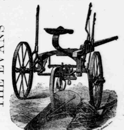
Made by the Moline Plow Company. Is the only entirely wrought-iron adjustable frame made, can be used with any sized plow, and is adjustable to all kinds of ground, having a lever on either side:
