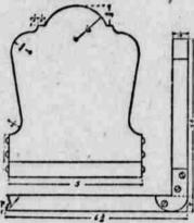
Use %-inch stock to make it. You will find a good size is 13 1/2 inches long. The two hinges should be exactly alike of sheet brass. When your rack is finished smooth it all over carefully, rub down, stain or paint any color you wish.
