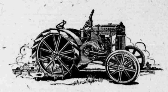
This machine weighs but 5,500 lbs. and capable of pulling three 14-inch plows in any kind of soil.
