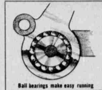
Ball bearings make easy running
