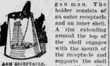
in position. The sides of the shell are spaced from the wall of the receptacle, the sides of the the receptacle converge. The bottom of the inner receptacle is perforated. Cigar or elgarette ashes dropped into the holder drop through the perforntions into the lower receptacle. If the holder is knocked over, which very frequently happens, the ashes are prevented from falling on the floor and injur-
